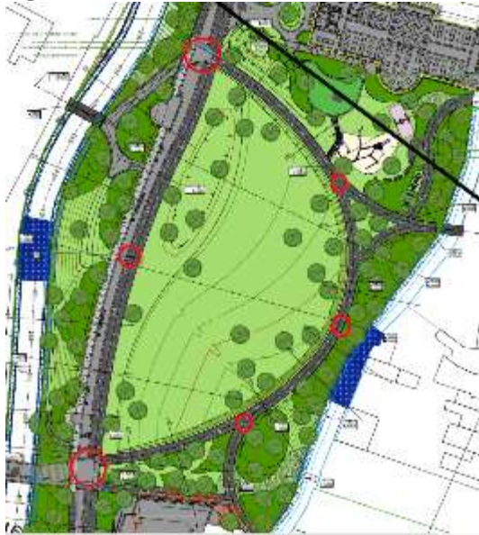
Figure 2: possible locations for traffic sensors
